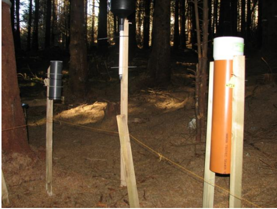
Figure 2 National throughfall collector (left) and EU standardized throughfall collector (right) at Ballinastoe intensive plot.
