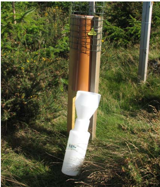
Figure 3 EU standardized throughfall collector at the control site at Ballinastoe. Collector consists of a 5L bottle with funnel attached and supporting field structure.
